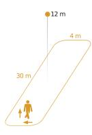
Possible mounting height: 4,00 m - 16,00 m Orange: radial and tangential
